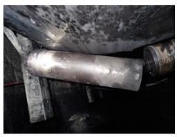
Mine operators must have systems to identify and change-out defective conveyor rollers. Workers conducting conveyor inspections must be aware of the increased risk of roller failure at high tension areas of conveyors. They must also diligently inspect for fire risks such as accumulation of material, failing or collapsed idlers and contact between conveyor belts and fixed structures.
