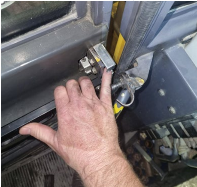
Figure 3: Showing where the fitter's fingers were placed in the door
