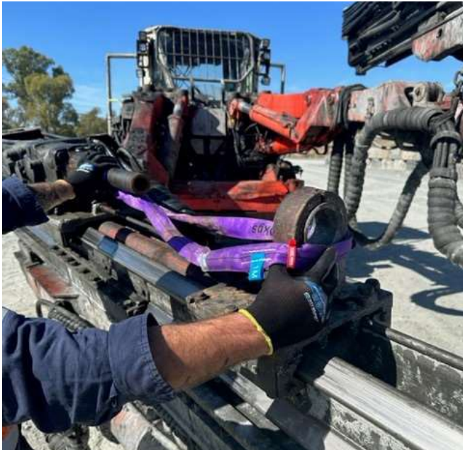
Figure 2: A simulation of where the fitter's thumb was caught
