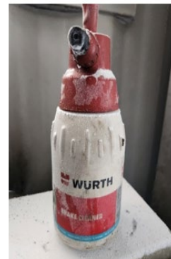
Figure 3 Brake cleaner handpump
