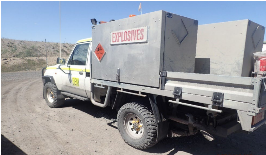
Figure 2: Typical shot firing vehicle – carry box – segregation
