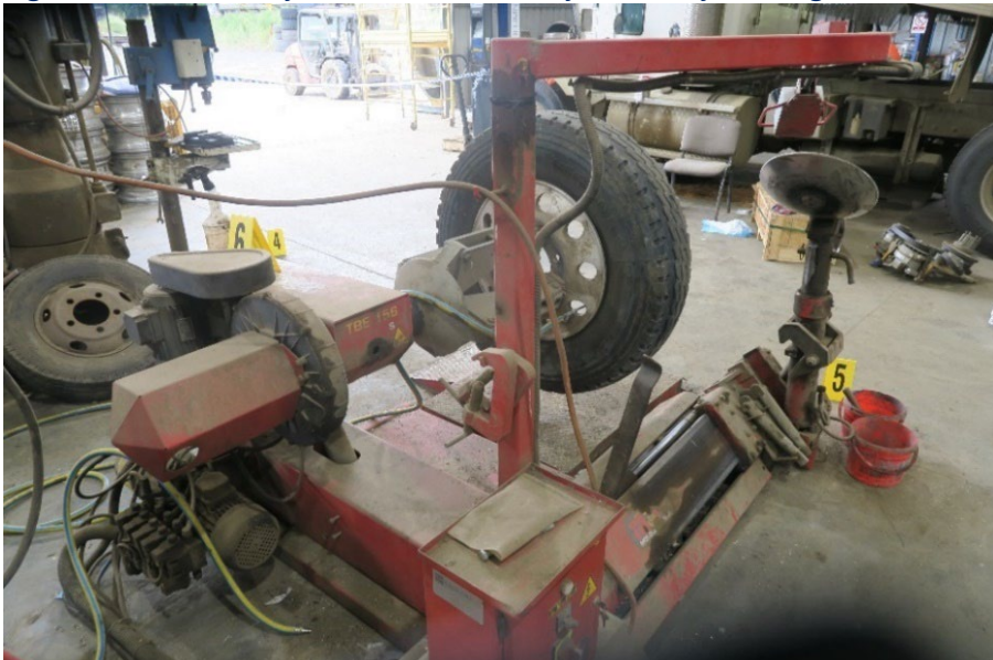
Figure 2: Rear view of tyre and wheel assembly fitted to tyre-fitting machine after the incident
