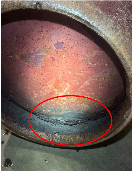
Figure 2: Underside of acetylene cylinder with heat affected area
