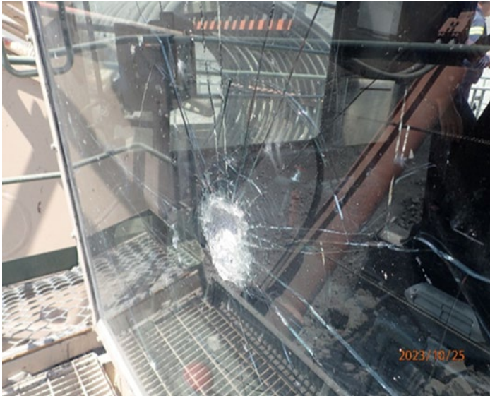
Figure 3: Inside the excavator cabin showing flyrock impact to windscreen and the position of the dozer after the incident
