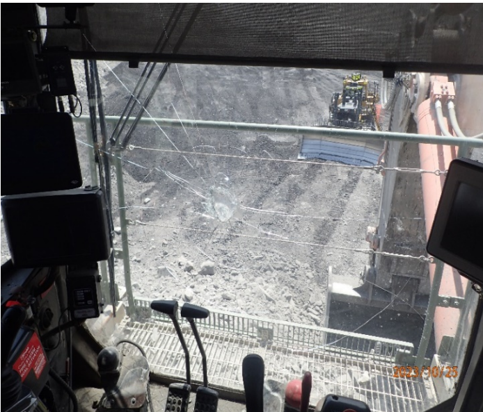
Figure 3: Inside the excavator cabin showing flyrock impact to windscreen and the position of the dozer after the incident
