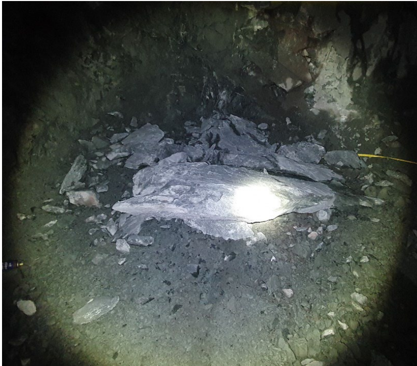
Figure 2: The slab of rock that hit the Jumbo operator
