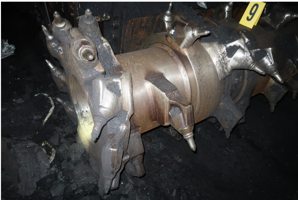
Figure 2 - Picks on the cutting drum of continuous miner, which are believed to have contacted a rock or similar material in the heading to provide an ignition source
