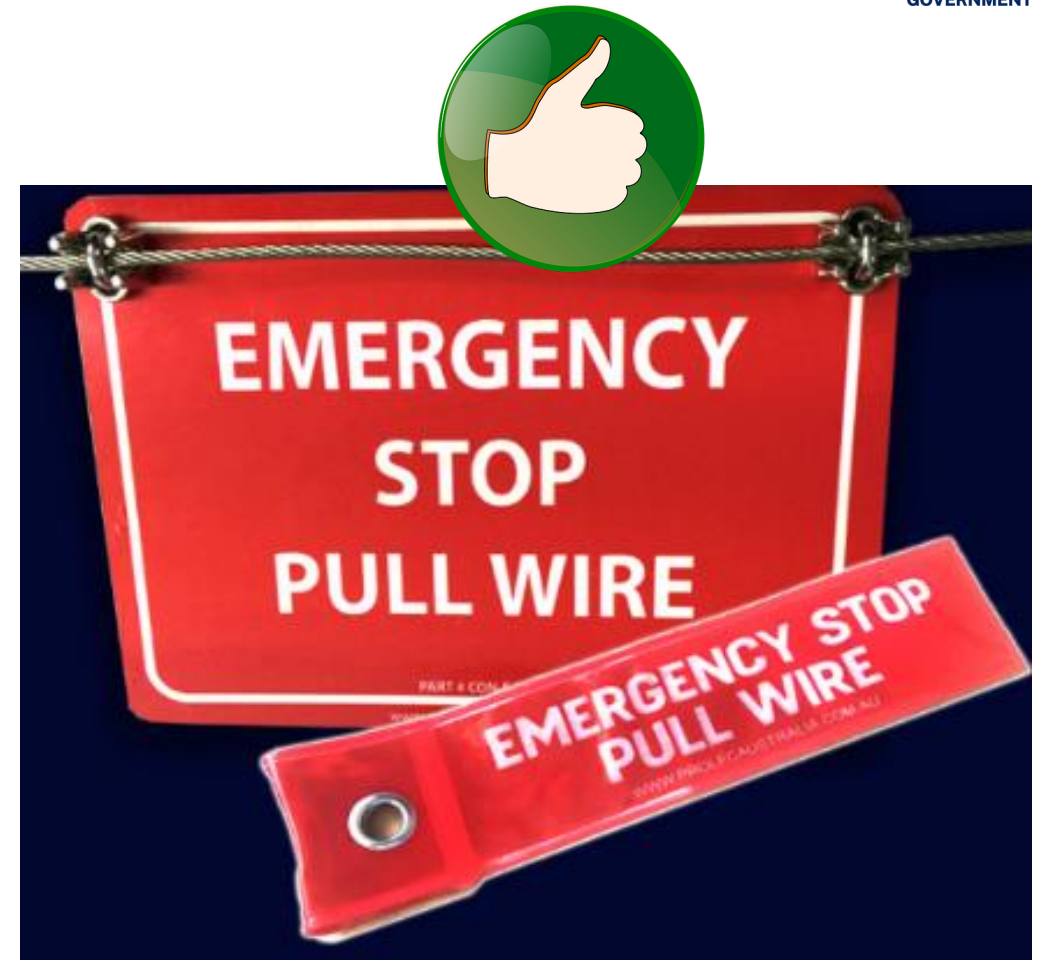
Types of signage for emergency stop lanyards
