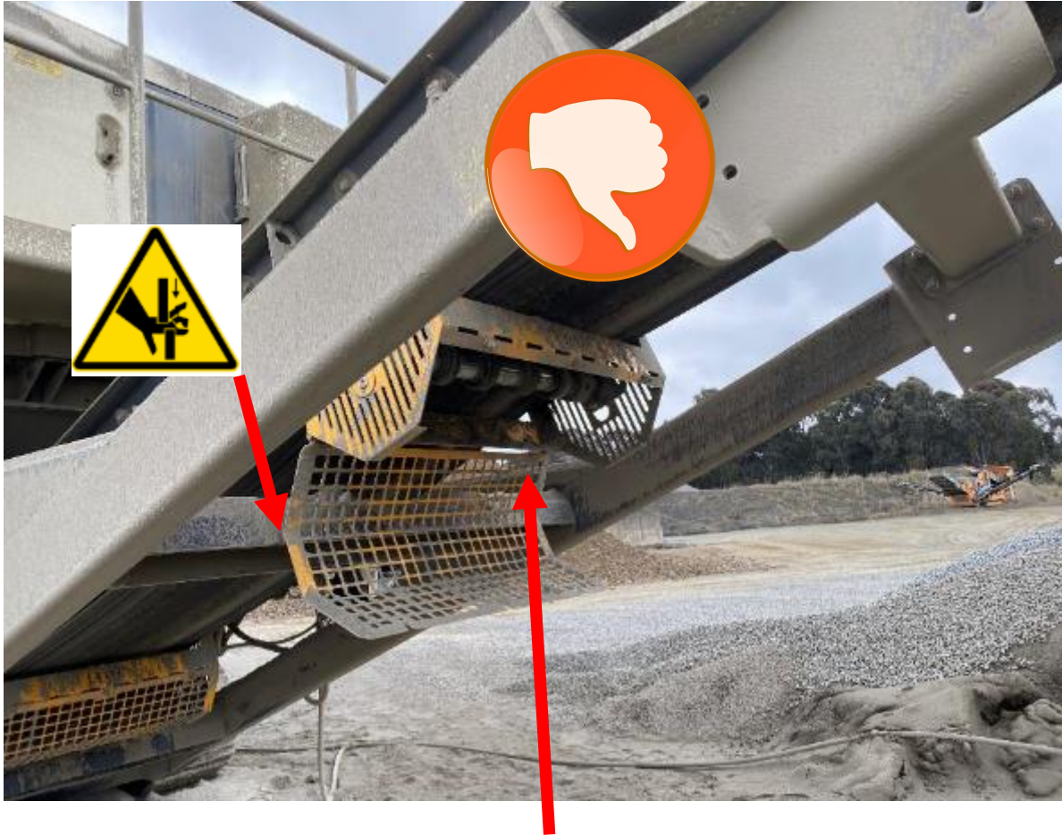
Hinged guard to assist in cleaning (but what if it was hinged on the opposite side? Hint: pinch point)
