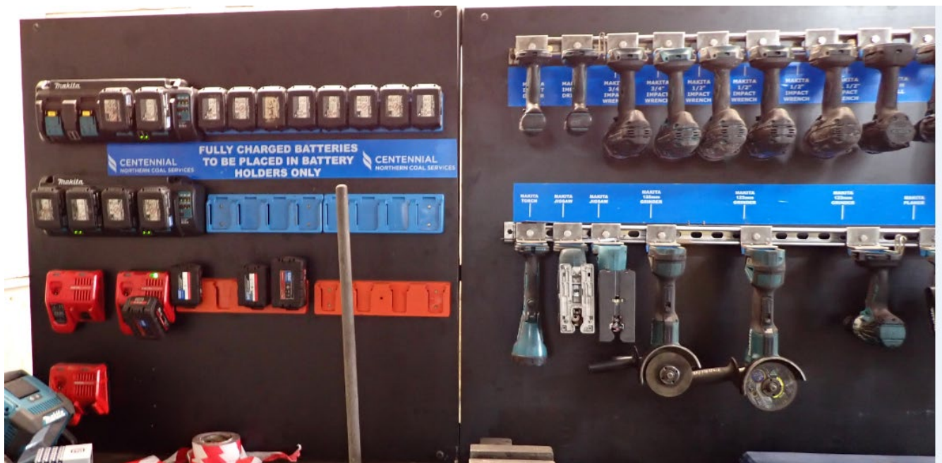
Figure 3 - Example of a well laid out charging station
