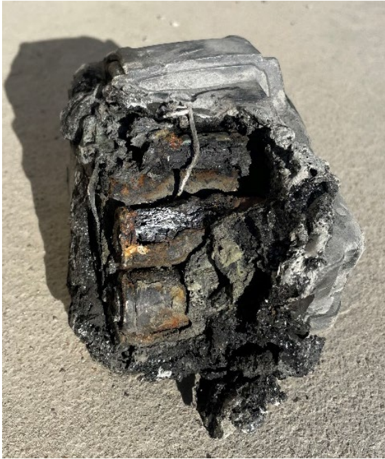
Figure 1 - Damage to battery after being run over
