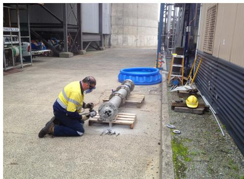
Figure 40: Photo of the dismantled adsorption column from the prototype test unit
