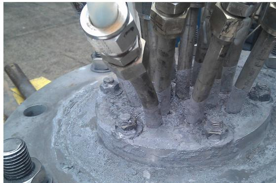
Figure 13: Modified regeneration tubes setup for the adsorption column in the prototype test unit
