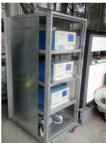
Figure 31: Individual analysers for measuring SO<sub>2</sub>, NO<sub>x</sub> and CO used for the solid sorbent CO<sub>2</sub> capture site trial
