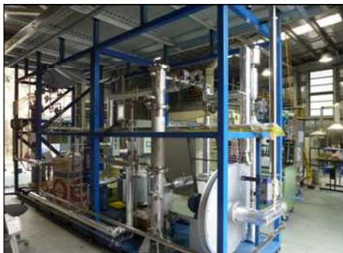
**Figure 18: The fully constructed large scale honeycomb carbon fibre composite CO<sub>2</sub> capture prototype test unit at QCAT.**
