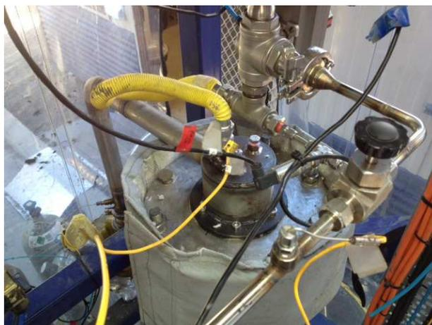
Figure 43: Photo of the redesigned regeneration set-up with welding of regeneration tubes at the top of the adsorbent column
