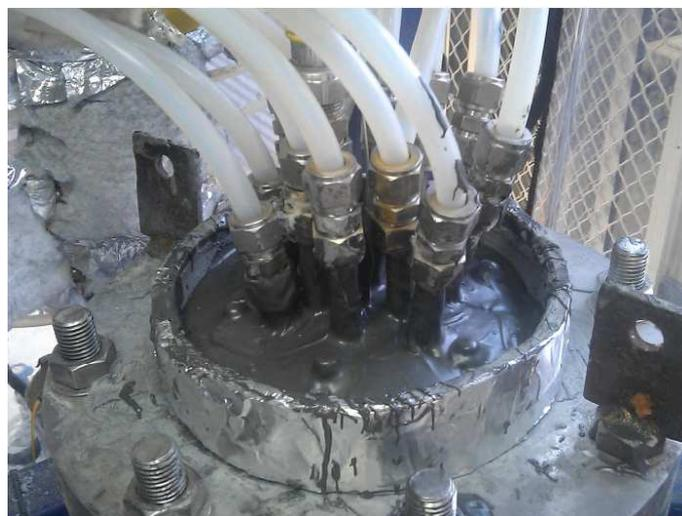
Figure 37: Photo of column resealing with high temperature epoxy sealant
