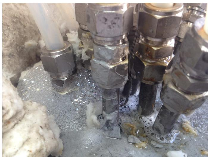
**Figure 36: Photo showing the gas leaking from the adsorption column**
