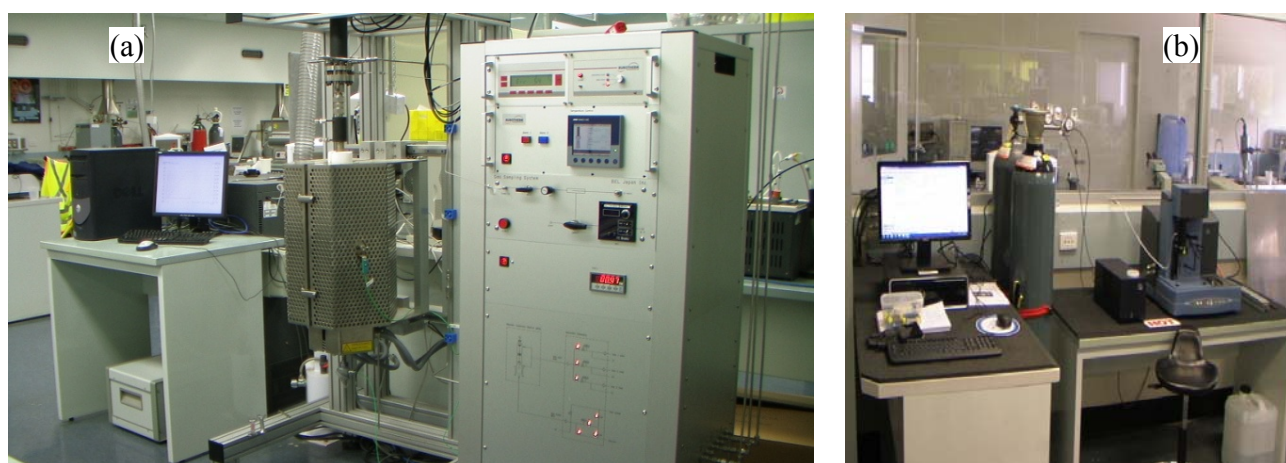
Figure 9: TGA units; (a) Rubotherm pressurised MSB-Aus-2004-00188 unit and (b) TA Instruments Q50 unit.
