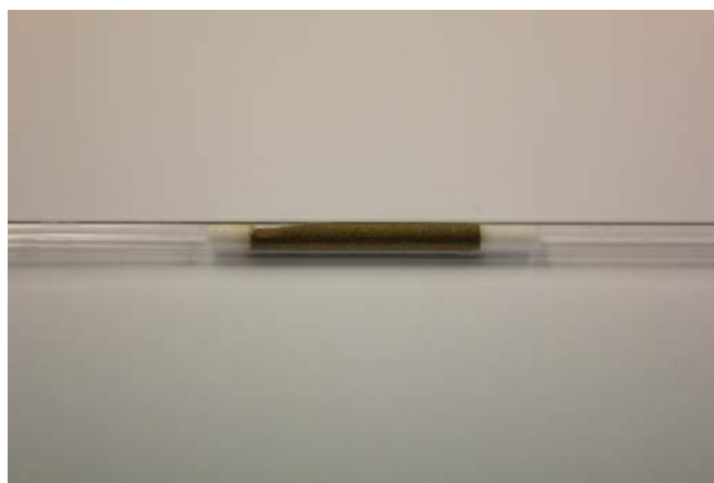
Figure 48: Photograph of the quartz tube reactor loaded with a metal oxide sample.
