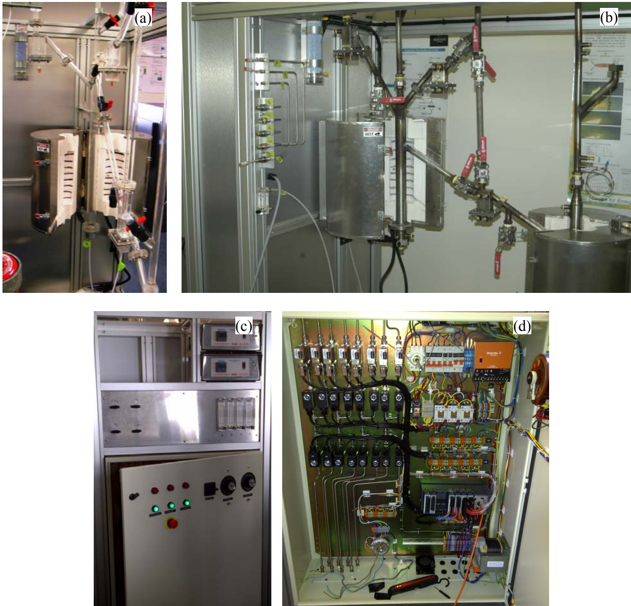
Figure 11: Pilot plant; (a) Perspex version; (b) SS version, (c) control box and (d) internal view of the control box.
