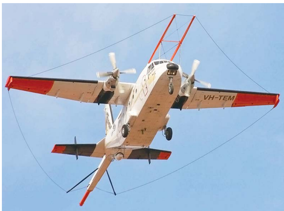
A fixed-wing aircraft with the AEM transmitter inside the aircraft and the receiver loop fixed to the outside (Source: CGG).
