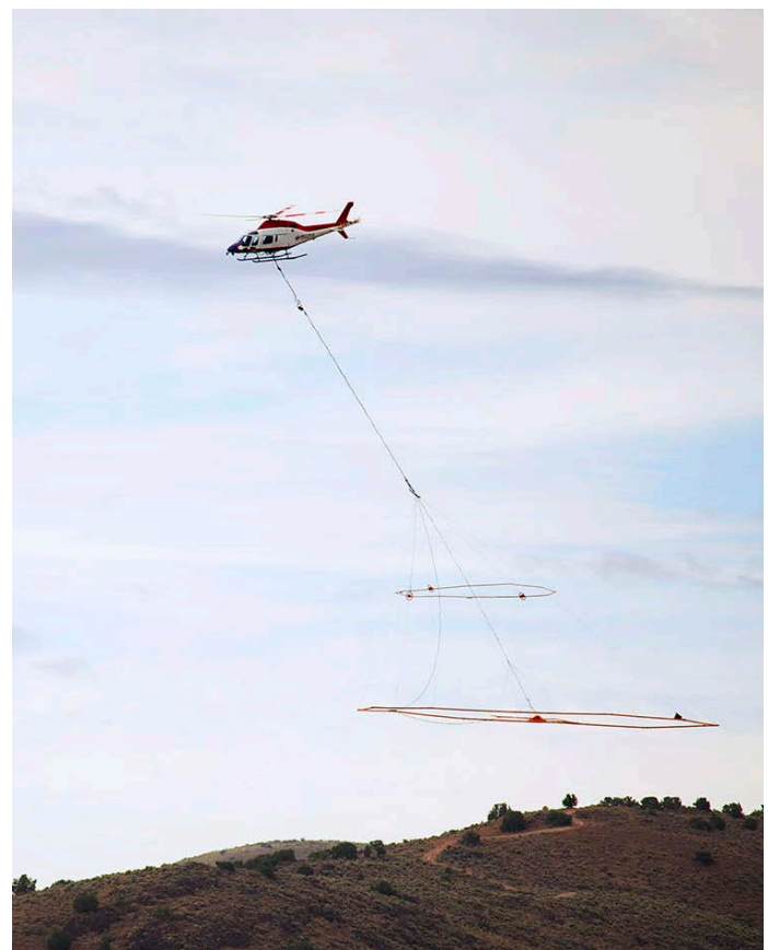
A helicopter towing an AEM transmitter and receiver (Source: Geotech Airborne).
