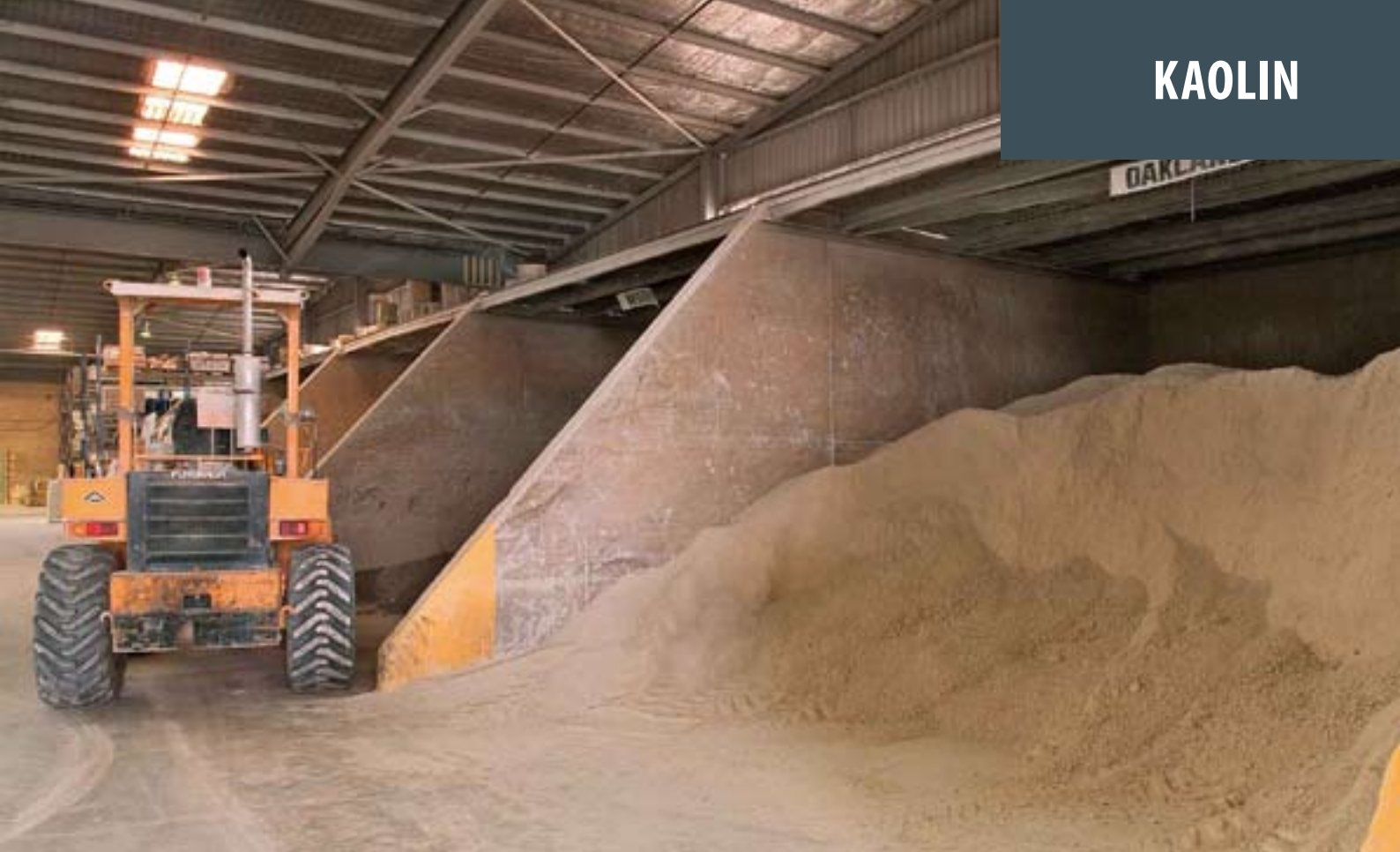
Photograph 9. Stockpile of raw kaolin, Caroma Industries ceramics plant, Sydney. This material came from kaolin deposits in the Oaklands–Coorabin area, southern New South Wales. The whiteness, plasticity and chemical stability of kaolin allow its use as a filler, extender, ceramic raw material, and pigment in coated films for paper manufacture. Kaolin is also an important raw material to refractories, and to catalyst, cement and fibreglass, industries. (Photographer D. Barnes)
