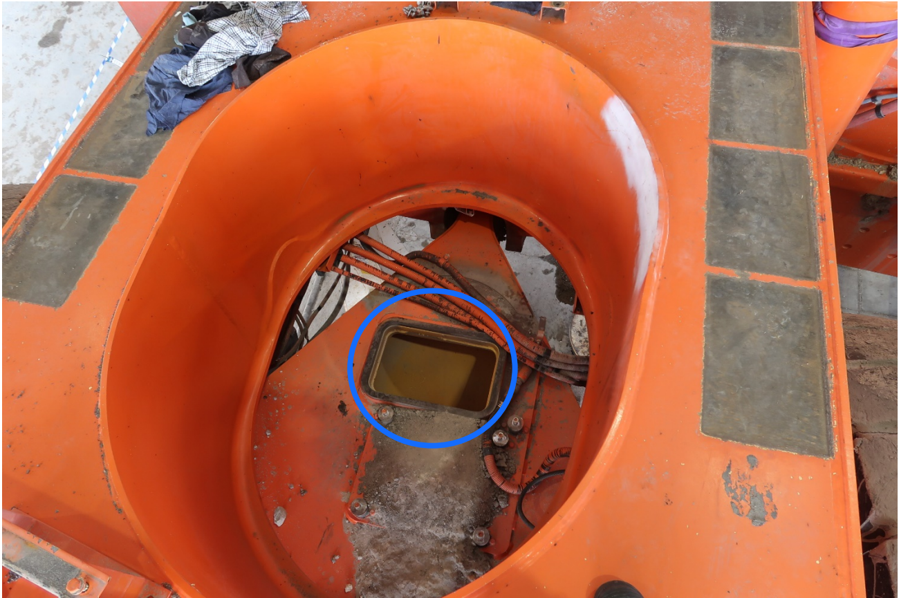
Figure 2 The lifting plate found after the incident on the cabin walkway
