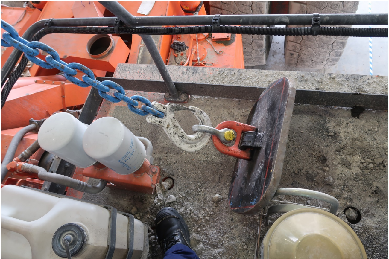
Figure 2 The lifting plate found after the incident on the cabin walkway
