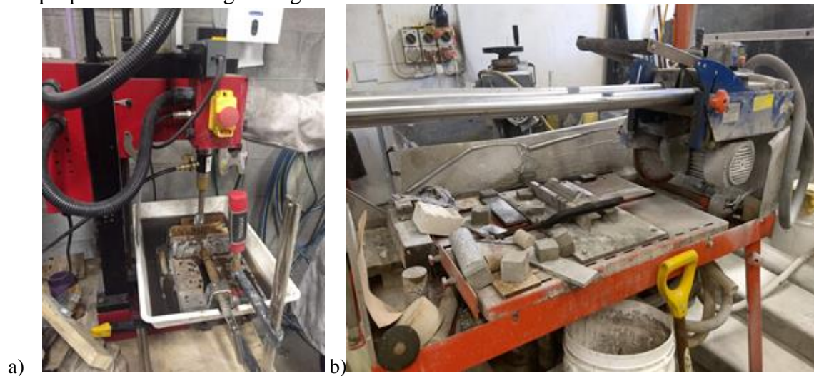
Figure. 1 Equipment used to prepare the cement samples: a) coring and b) cutting machines.
