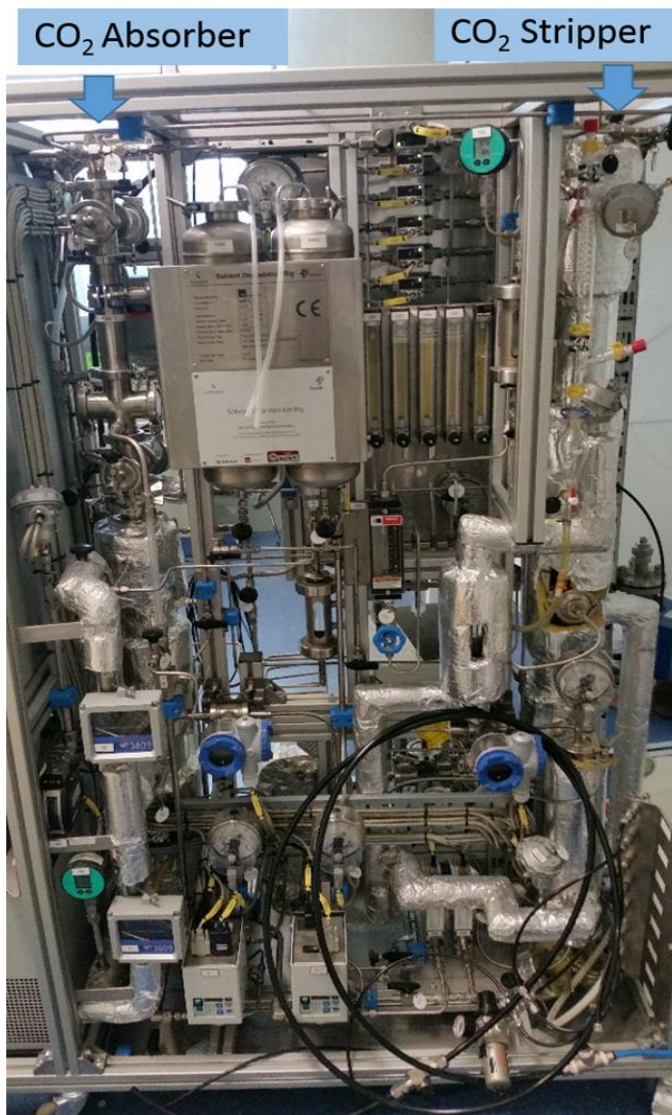
Figure 2 Solvent-degradation rig – standard configuration used for undertaking degradation studies
