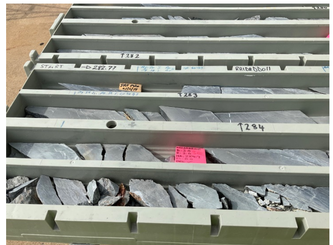
Figure 4 Example of core storage trays
