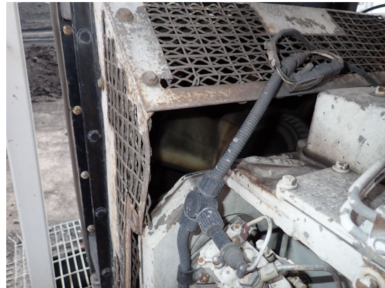
Figure 4– Ineffective guarding against rotating parts
