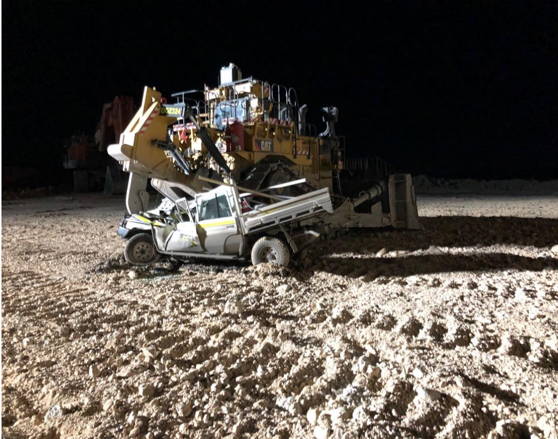
Failure to park vehicle safely
