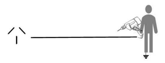
a) Draw an equivalent circuit showing the electric shock current flow paths through the human body and via the protective earth. (1 Mark)
