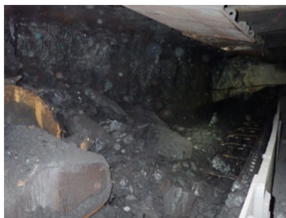
Below: Debris at the face after the coal burst.
