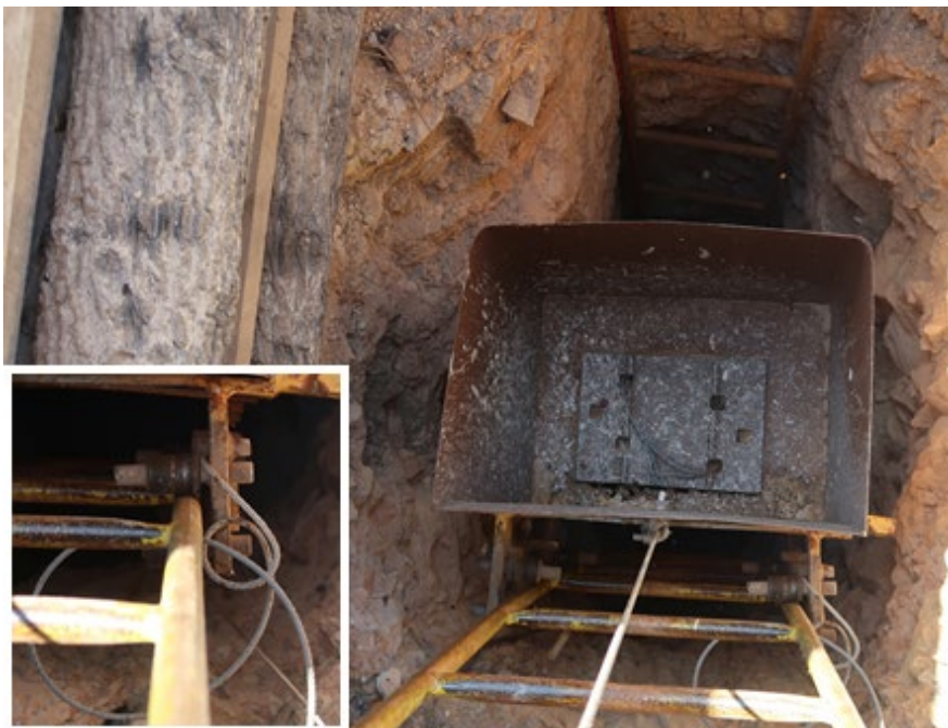
Figure 15: Entanglement of the bucket guide wheel with the engagement lever wire
