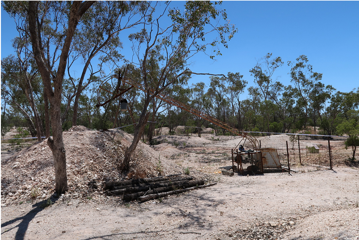
Figure 7: Hoist and opal dirt pile
