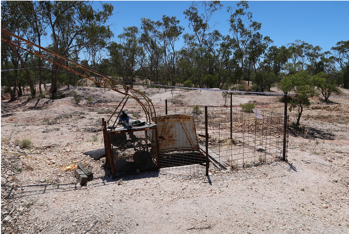
Figure 4: Hoist machinery cage and perimeter fencing around the hoist shaft
