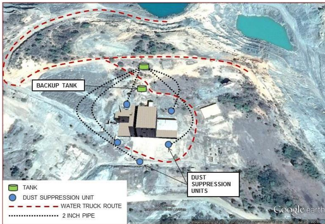
Figure 6 – Dust Suppression Water System.
